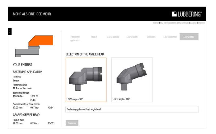
Select a LÜBBERING angle head L.SP3 angle in 90° or 110° and no adapter is needed.
